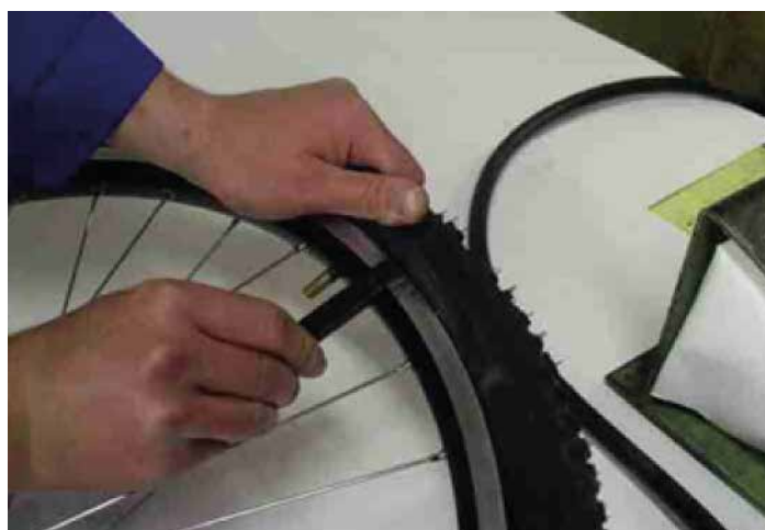
INCORRECT INSTALLATION / DISASSEMBLY
